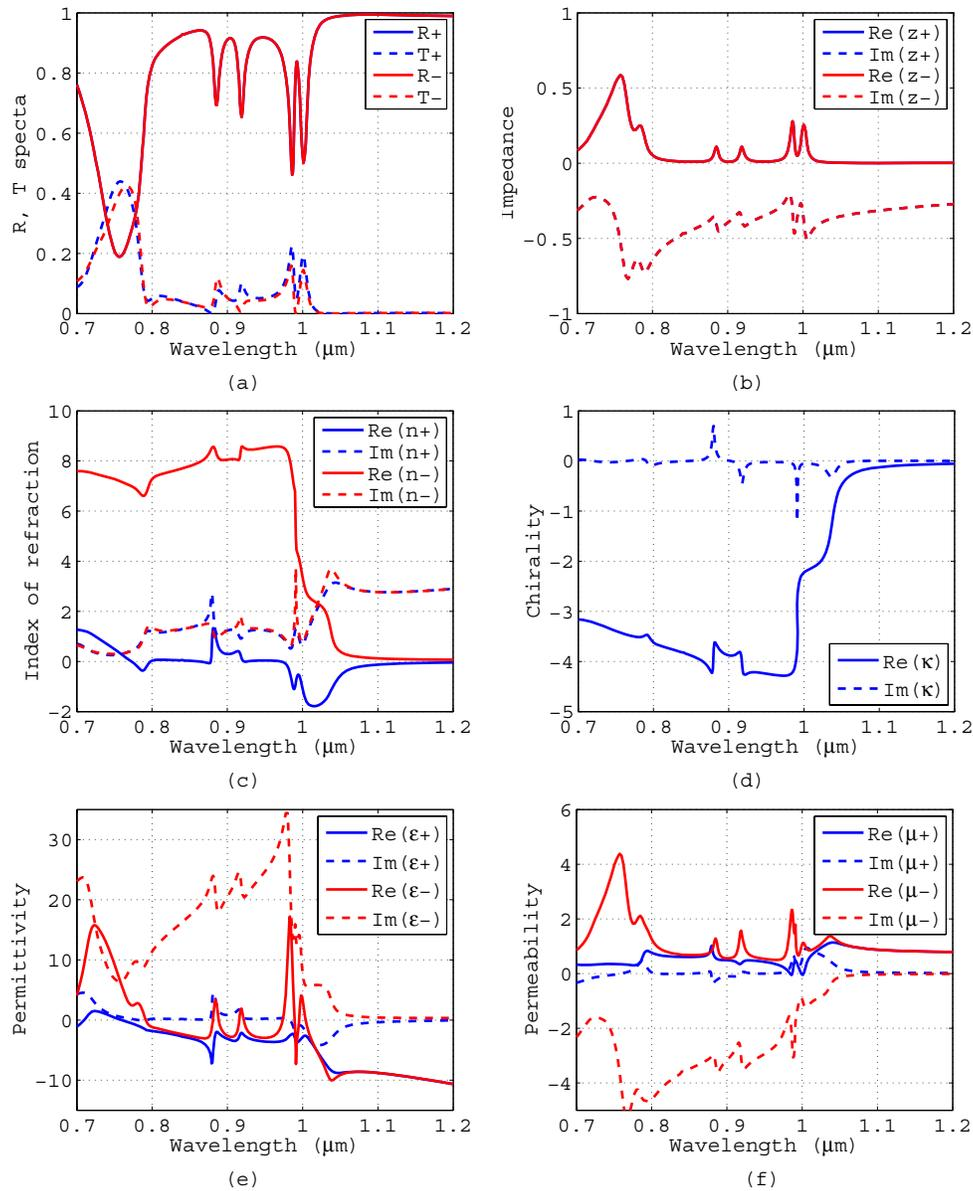
Fig. 3. (Color online) The spectra and material parameters of the chiral optical metamaterial: (a)  $R_{\pm}$  and  $T_{\pm}$  (reflectance and transmittance), (b)  $z_{\pm}$ , (c)  $n_{\pm}$ , (d)  $\kappa$ , (e)  $\epsilon_{\pm}$ , and (f)  $\mu_{\pm}$ .
