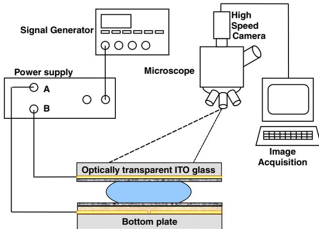
**Figure 5.** Schematic of the experimental setup used for the measurement of droplet velocities.
