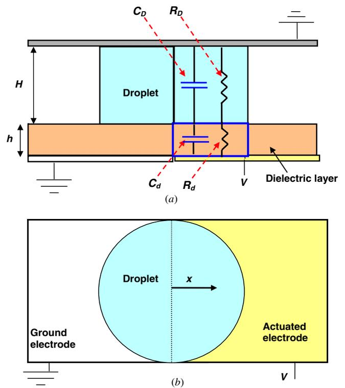
Figure 2. Schematic illustration of a droplet at the midpoint of the transition: (a) side view and (b) top view.
