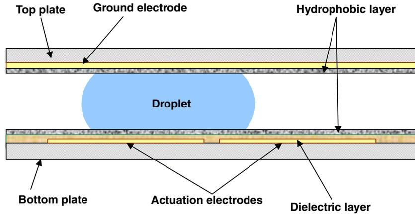
Figure 1. Representative device for electrical actuation of droplets [10].
