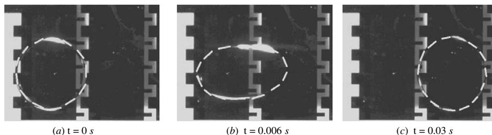
**Figure 6.** Transition of a 2 mm diameter  $10^{-3}$  M KCl droplet under an ac voltage of magnitude 50 V and frequency 50 Hz; the outline of the droplet has been highlighted with a dashed line for easier recognition; (a)  $t = 0$  s, (b)  $t = 0.006$  s and (c)  $t = 0.03$  s.
