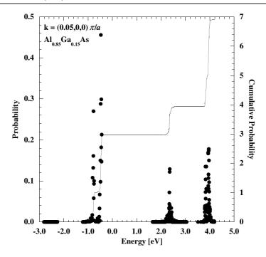
**Figure 1.** Probability (symbols) and cumulative probability (solid line) versus supercell-eigenstate energy,  $E_p$ , for the  $40 \times 2 \times 2$  Al<sub>0.85</sub>Ga<sub>0.15</sub>As random-alloy supercell at  $\mathbf{K} = \mathbf{0}$ ,  $\mathbf{k} = \mathbf{G} = (0.05, 0, 0)\pi/a$ . Here the algorithm could resolve a state at about 2.46 eV.
