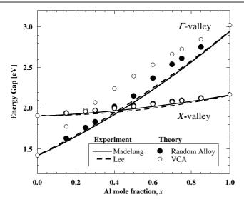
**Figure 3.** Band gaps versus mole fraction for  $Al_xGa_{1-x}As$ . Solid circles: gaps based on states projected out of the  $40 \times 2 \times 2$   $Al_xGa_{1-x}As$  random-alloy supercell; open circles: gaps determined from the VCA bands; solid lines: experimental results from Madelung [17]; dashed lines: experimental results from Lee *et al* [20]. Note the significantly better agreement of the random-alloy results with experiment.
