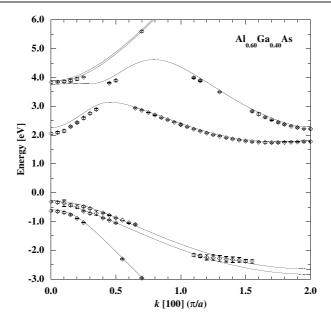
**Figure 2.** Approximate bands with error bars projected out of the  $40 \times 2 \times 2$  Al<sub>0.60</sub>Ga<sub>0.40</sub>As random-alloy supercell (diamonds) and the VCA bands (solid lines) for bulk Al<sub>0.60</sub>Ga<sub>0.40</sub>As. Note the significantly lower conduction-band minimum at  $\mathbf{k} = \mathbf{0}$  in the random-alloy case.
