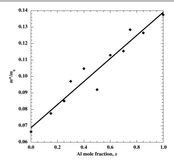
Figure 4. Approximate Γ-valley effective masses versus mole fraction for  $Al_xGa_{1-x}As$ . Solid symbols: approximate masses based on states projected out of the  $40 \times 2 \times 2$   $Al_xGa_{1-x}As$  random-alloy supercell; solid line: best linear fit to the data.
