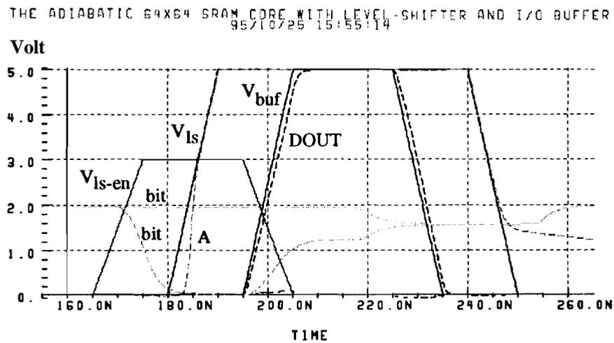
Figure 11: Waveforms for the adiabatic level-shifter
