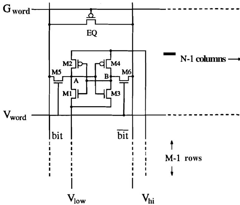
Figure 5: Another memory core organization.  $V_{hi}$  and  $V_{low}$  run vertically and are generated by column driver circuitry. In this core organization, only selected columns are activated.
