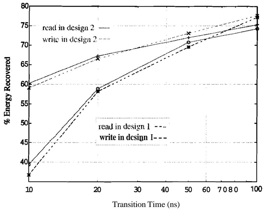
Figure 15: Energy recovery in adiabatic memory core
