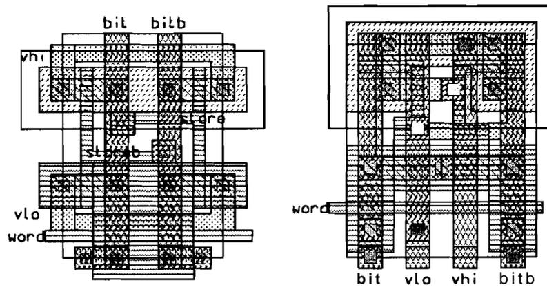
Figure 14: Layout of two *SRAM* cell configurations. The cell shown on the left side is for row activated memory core organization, and the cell shown on the right side is for column activated memory core organization, in which only the selected columns are active. The supply lines  $V_{hi}$  and  $V_{low}$  run horizontally in the left cell and vertically in the right cell.
