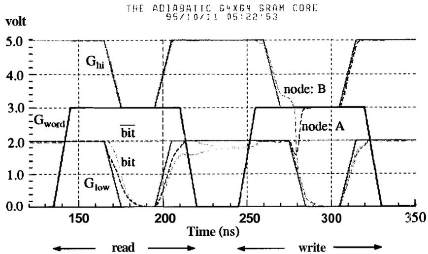
Figure 7: Waveforms for the SRAM core
