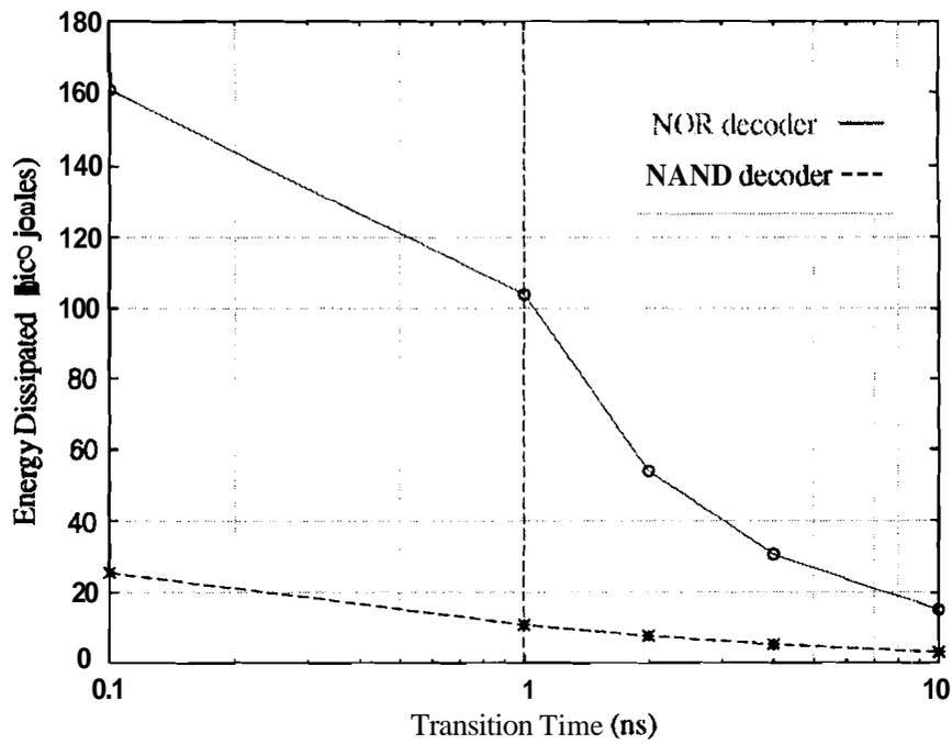
Figure 18: Comparison of energy dissipation in adiabatic NAND and NOR decoder
