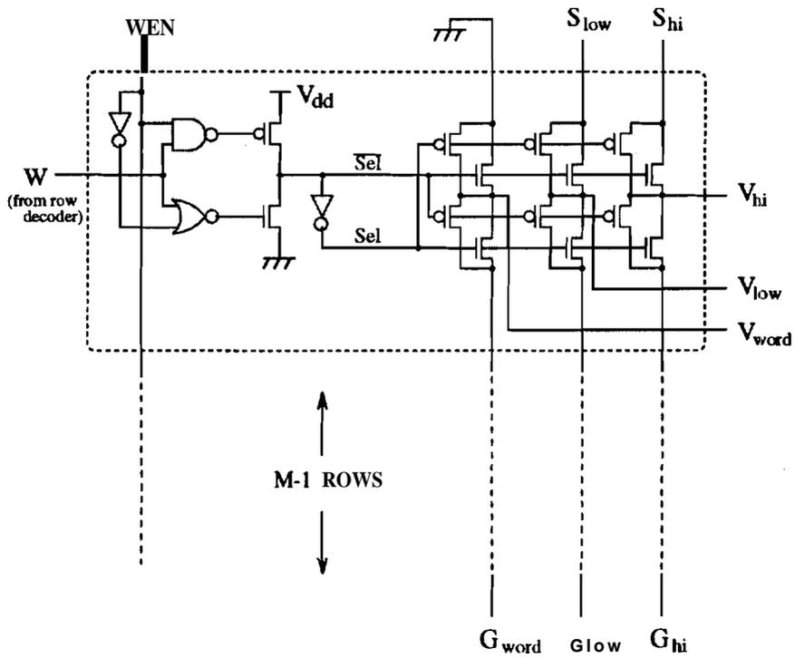
Figure 6: The row driver circuit
