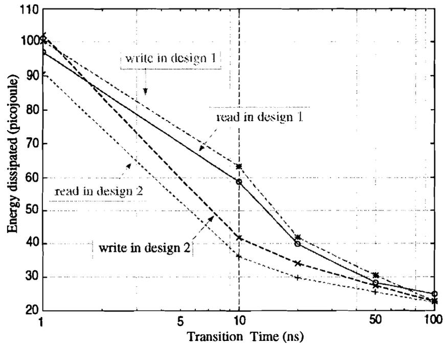
Figure 16: Comparison of energy dissipation in two memory core organizations
