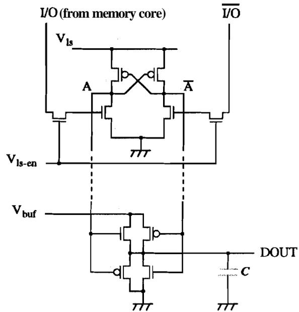
Figure 10: Adiabatic level-shifter and I/O buffer
