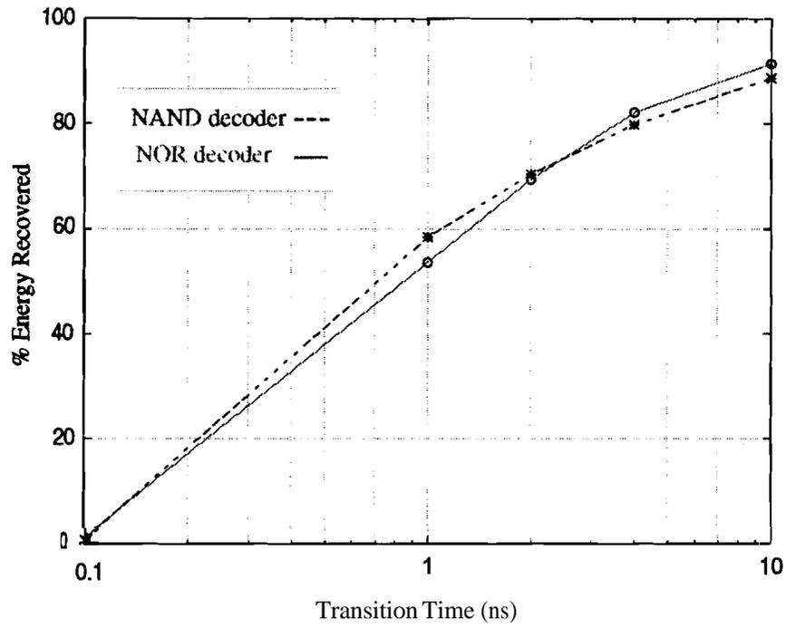
Figure 17: Energy recovery in 6-to-64 adiabatic NAND and NOR decoders
