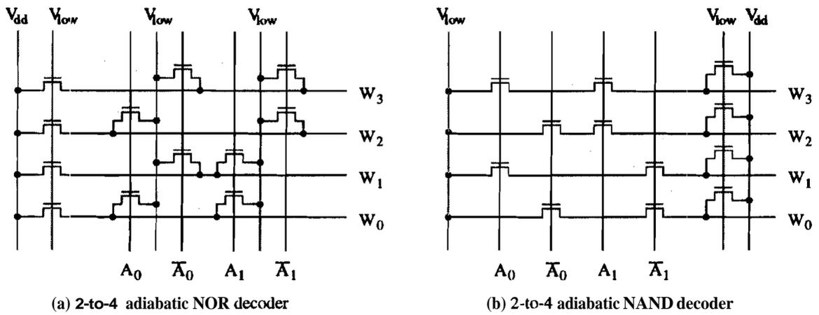
Figure 8: Configurations of adiabatic address decoder
