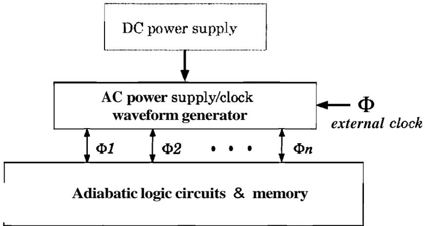
Figure 2: A framework for power supply and circuit
