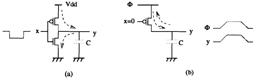
Figure 1: Charging and discharging in standard CMOS and adiabatic fashion
