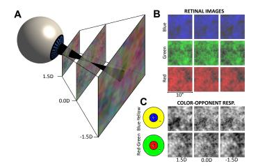
Figure 1: A. Longitudinal chromatic aberration (LCA), and B. the associated retinal images with positive, zero, and negative defocus, together with C. the Blue-Yellow and Red-Green color-opponent responses.
