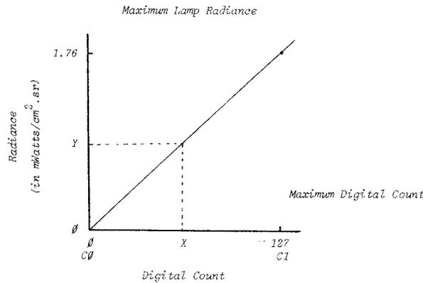
Figure 3. Graphic Representation of the "Linear Calibration" of Landsat 1, Band 6 data.
