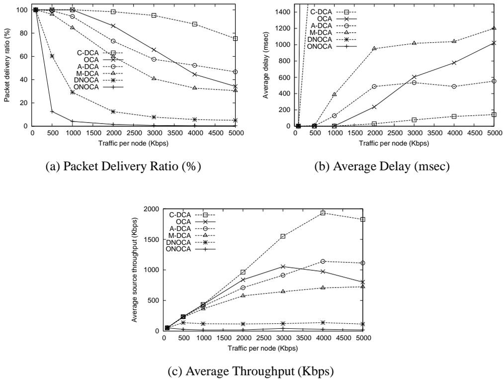
Figure 7: Comparison of different mesh network architectures.
