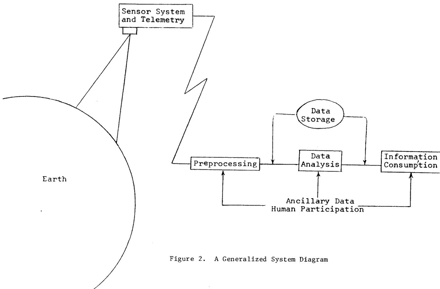
Figure 2. A Generalized System Diagram
