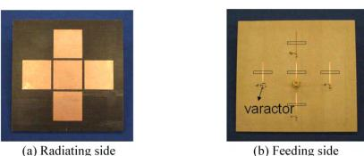
Fig.2 Fabricated parasitic patch array
