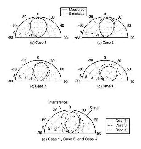
Fig.3 Tunable radiation pattern for different reactive loads
