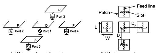
(a) Driven and parasitic patch array
