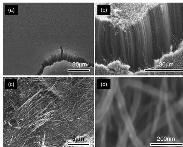
**Figure 1.** FESEM images of MWCNTs grown from 1Fe@den catalysts calcined at 550 °C. (a) low-resolution image showing the large and uniform coverage of MWCNTs; (b) vertical orientation of the MWCNTs; (c) the substrate after scratching; and (d) high-resolution image of MWCNTs.
