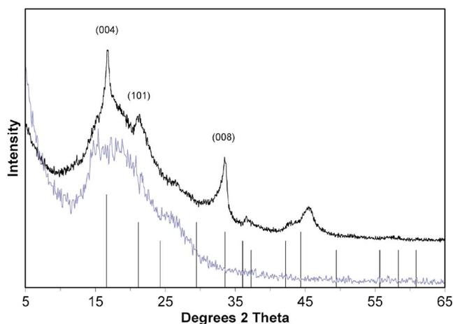
FIG. 2. (Color online) Powder XRD scan ( $\text{Cu } K\alpha$  radiation) of a Stage-1 ( $\text{KC}_8$ ) herringbone GCNF-potassium metal intercalate [top curve, peaks indexed to corresponding peaks of bulk  $\text{KC}_8$  shown as a line pattern (JCPDS Card 04-0221)] recorded under a protective Kapton™ cover. An XRD scan typical of the Kapton™ cover film is shown as the bottom curve, and a slight sample-displacement offset is evident.
