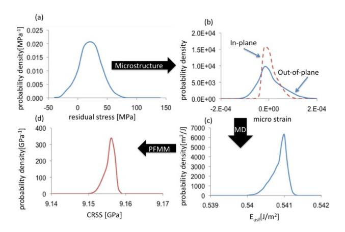
Figure 3.3: Uncertainty propagation across scales. The experimental distribution of residual stresses in the longitudinal direction of the membrane (a) is converted into a distribution of inplane and out-of-plane stress for each grain using the iso-strain approximation and XRD texture (b). The strains are then used with an MD response surface to predict the distribution of unstable stacking fault energies (c) that are used to predict a pdf of CRSS using PFMM response surfaces (d).
