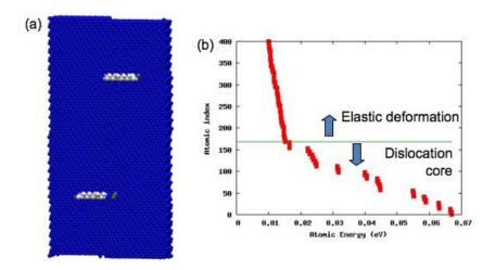
Figure 2.4: MD simulations of dislocations in Ni. (a) Atomic snapshot of two dissociated screw dislocations; light atoms denote stacking faults. (b) Atomic energy in decreasing order as a function of atom number for our relaxed simulation cell with two dissociated screw dislocations, each seven Burgers vector long; we define core as the 12 atoms with highest energy per dislocation, per Burgers vector.
