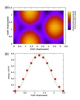
Figure 2.5: Gamma surface of Ni at T=300 K. (a) 2D map of the energy per unit area as two blocks are displaced in the (111) plane. (b) Energy per unit area for a displacement along the [110] direction; squares show MD results and the line is a fit of the function used in the PFDD model to the MD data.
