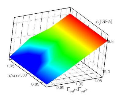
Figure 3.1: CRSS response function calculated from PFDD simulations as a function of the elastic energy and the unstable stacking fault energy.
