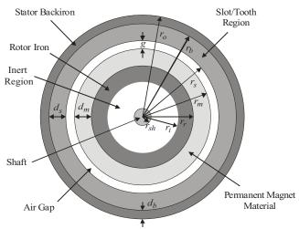
Fig. 3. PMSM Configuration.
