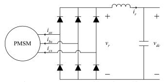
Fig. 5. System II. PMSM with passive rectifier.
