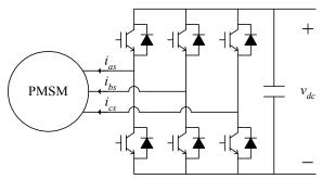
Fig. 2. System I. PMSM with active rectifier.
