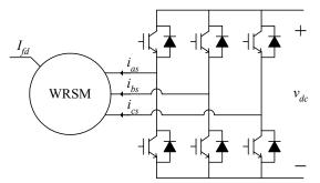
Fig. 6. System III. WRSM with active rectifier.
