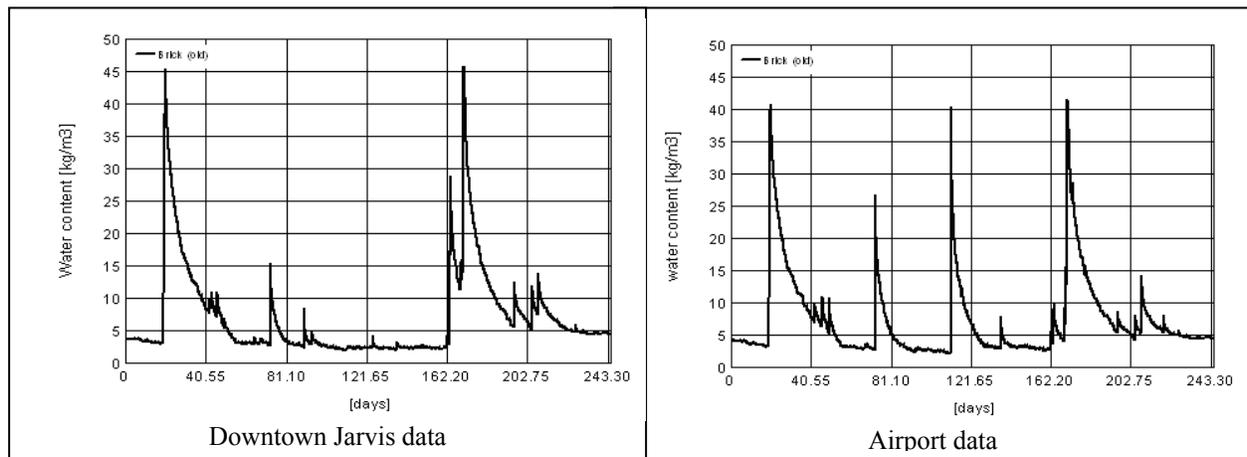
Figure 5: Moisture content of brick during 1978 (April 1, to November 30)
