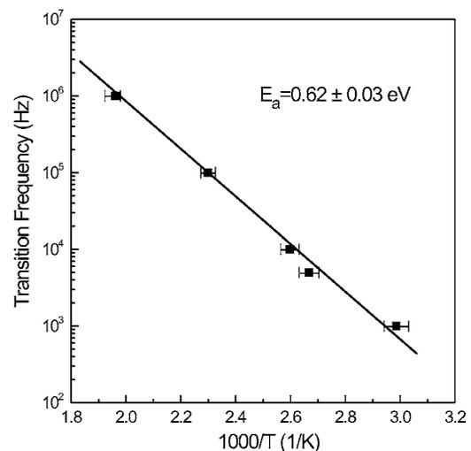
FIG. 3. Temperature dependence of the transition frequency between high and low frequency  $C$ - $V$  curves. Activation energy of the minority-carrier recombination is obtained from the slope of the linear fitting trace.
