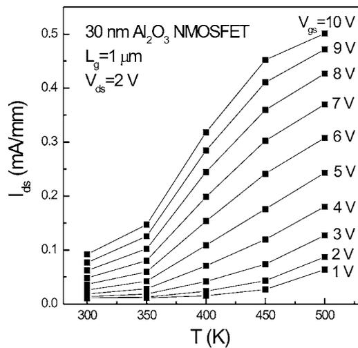
FIG. 4. Temperature dependence of the drain current at  $V_{ds}=2$  V of a  $1\ \mu\text{m}$  gate length inversion channel enhancement-mode InGaAs MOSFET with a 30 nm ALD  $\text{Al}_2\text{O}_3$  as a gate dielectric.
