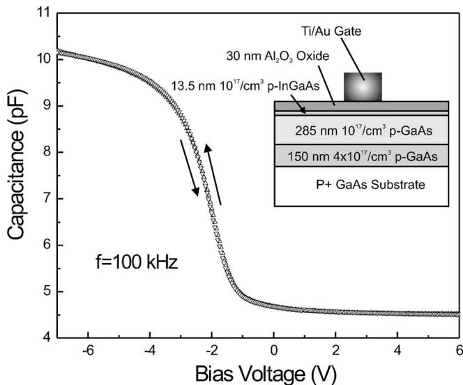
FIG. 1.  $C$ - $V$  characteristics of ALD  $\text{Al}_2\text{O}_3/\text{InGaAs}/\text{GaAs}$  MOS structure at an ac frequency of 100 kHz. The up triangles are the data taken from  $-7$  to  $6$  V; the down triangles are the data obtained from  $6$  to  $-7$  V. The area of Ti/Au electrode is  $4418 \mu\text{m}^2$  and the MOS capacitor was measured at room temperature. Inset: Cross section of an  $\text{Al}_2\text{O}_3/\text{InGaAs}/\text{GaAs}$  capacitor fabricated for this study.
