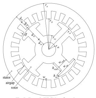
Fig. 7. Example WRSM configuration.
