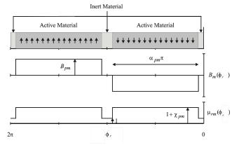
Fig. 4. Developed diagram of permanent magnet region.
