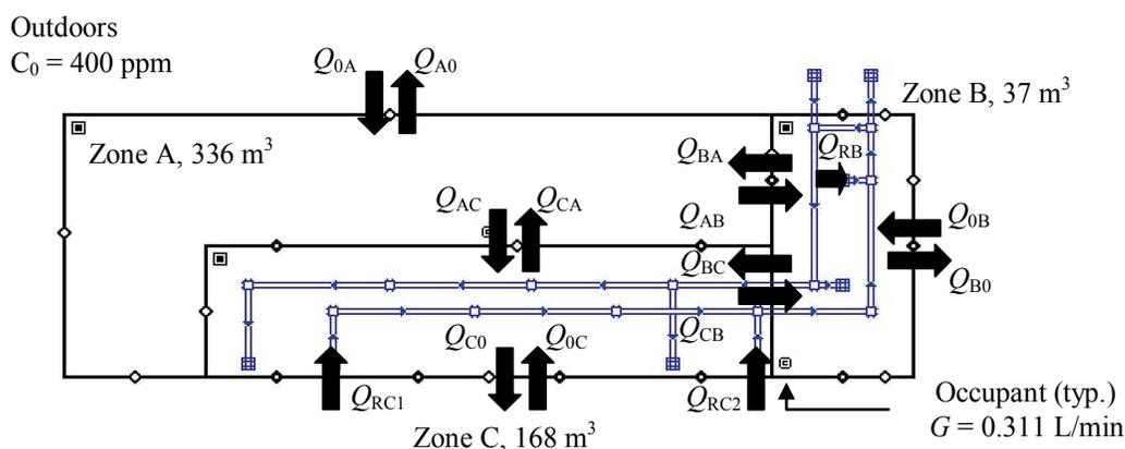
Figure 3: Building model showing parameters (airflow rates) estimated.
