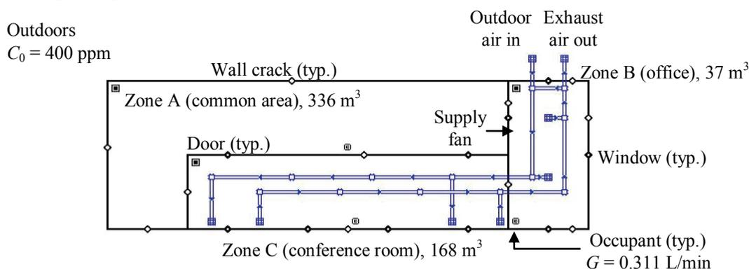
Figure 1: CONTAM model of three-zone test building.
