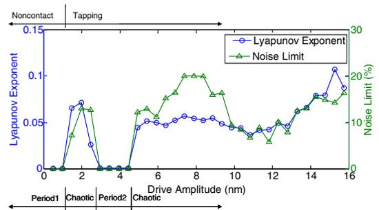
FIG. 1 (color online). Largest Lyapunov exponent and noise limit versus dither piezo driving amplitude for one of the Force Modulation ( $\omega_0 = 66.3$  kHz) microcantilevers in a dry nitrogen environment over freshly cleaved HOPG.
