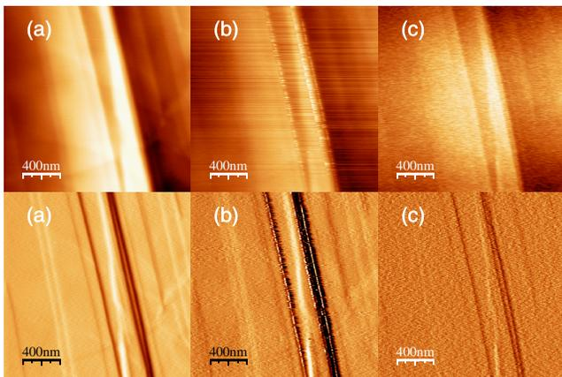
FIG. 3 (color online). Influence of chaotic tip oscillations on the nanometrology of a freshly cleaved HOPG surface. Topology map (top) and error map (bottom) with driving amplitudes of (a) 0.49 nm (period-1, noncontact regime), (b) 1.97 nm (chaotic, tapping regime), and (c) 14.76 nm (chaotic, tapping regime). The scan area is  $2 \times 2 \mu\text{m}^2$ .
