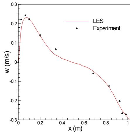
Figure 4b: Mean vertical velocity (w) with x at  $y=0.15\text{m}$  and  $z=0.52\text{m}$ .
