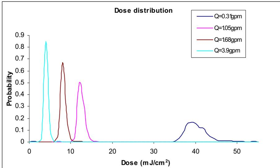
Figure 3. UV dose distribution estimates for operating conditions that correspond with physical tests of the prototype reactor.
