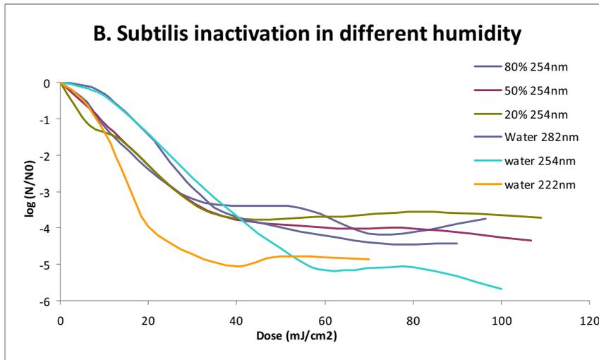
**Figure 4.** UV dose-response behavior for *B. subtilis* spores in gas-phase as a function of relative humidity.
