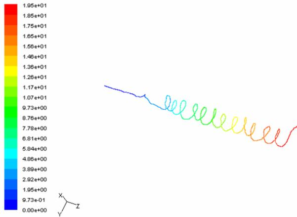
Figure 2. Particle trajectory in the reactor (velocity = 0.1638 m/s (0.31gal/min)).
