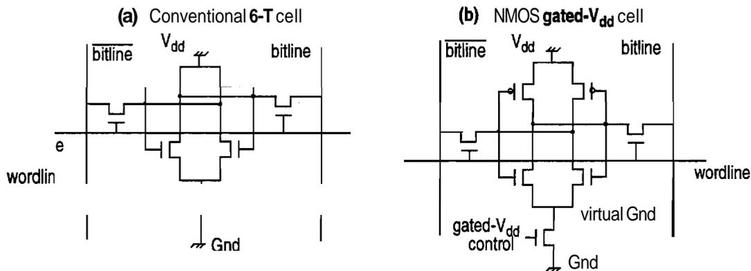
FIGURE 3: 6-T SRAM cell schematics: (a) conventional, (b) with NMOS  $\text{gated-}V_{dd}$ .
