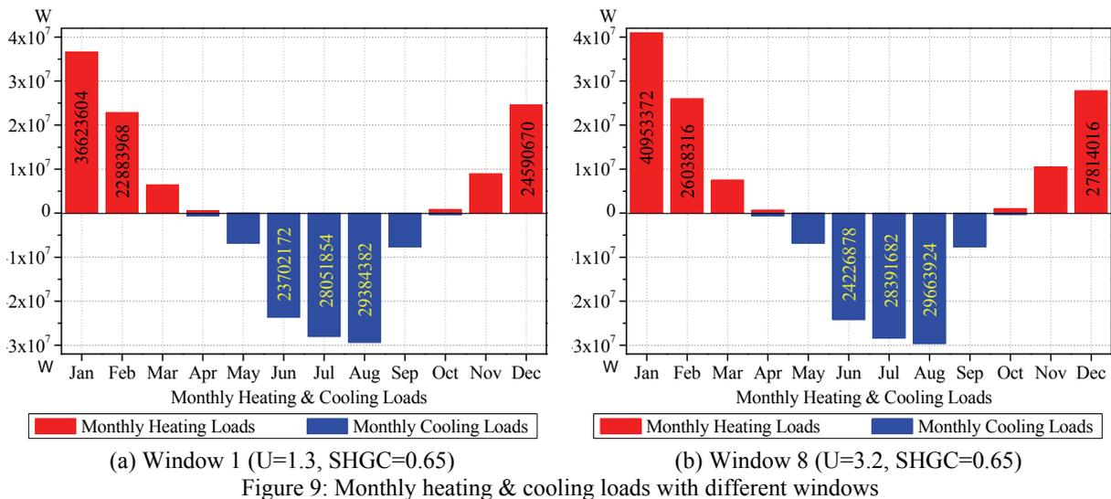
Figure 9: Monthly heating & cooling loads with different windows
