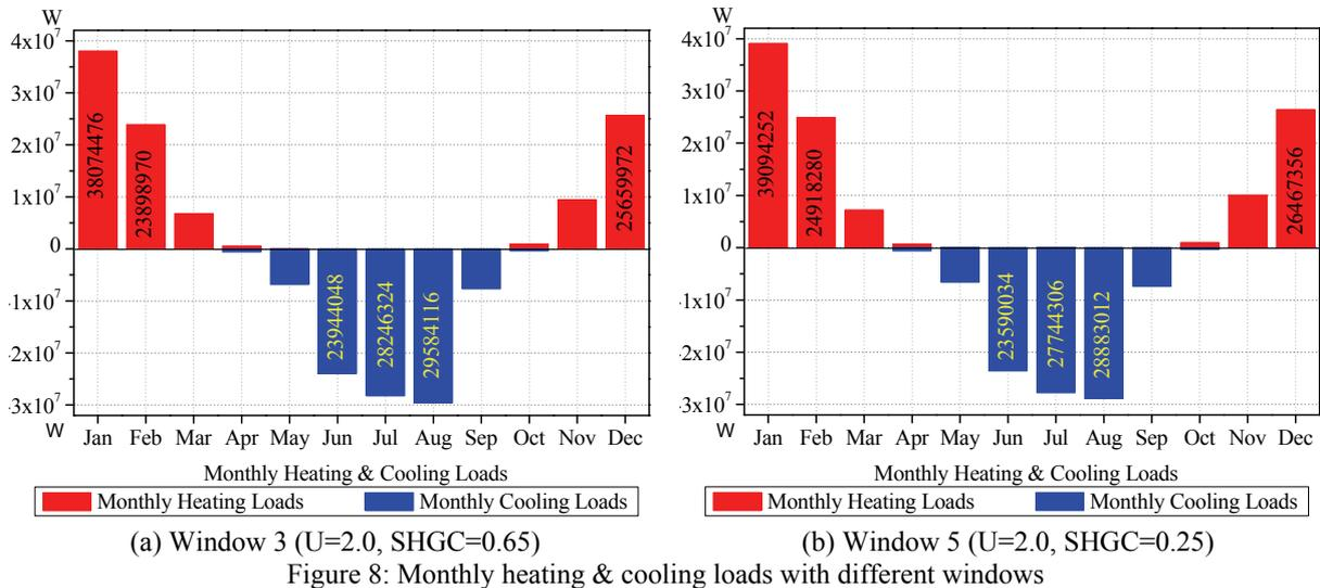
Figure 8: Monthly heating & cooling loads with different windows
