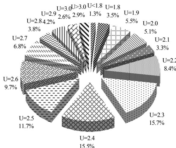
Figure 1: Distribution of U-factors of windows acquired energy efficiency labels (unit:  $W/(m^2 \cdot K)$ )
