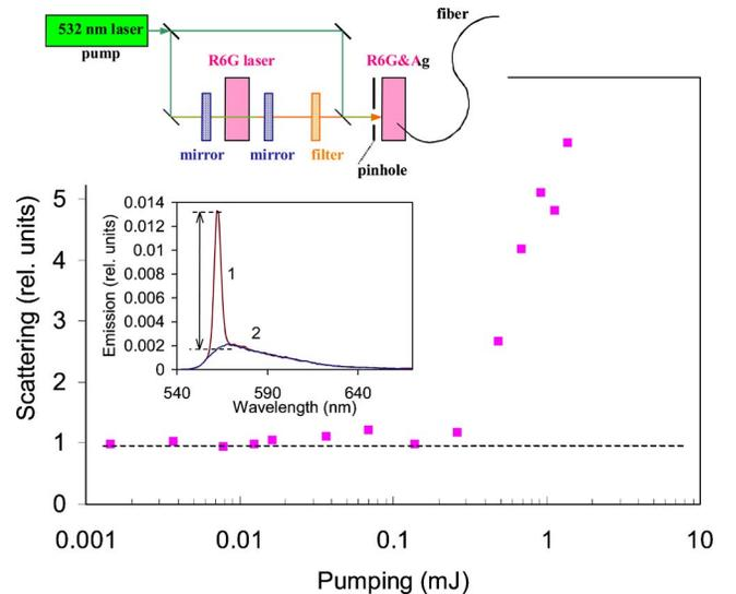
Fig. 1. (Color online) Intensity of the Rayleigh scattering as the function of the pumping energy, R6G,  $2.1 \times 10^{-5} \text{ M}$ ; Ag aggregate,  $8.7 \times 10^{13} \text{ cm}^{-3}$ . Upper inset: Pump-probe experimental setup for the Rayleigh scattering measurements. Lower inset: 1, spectrum of scattered light and spontaneous emission; 2, spectrum of spontaneous emission only. The difference between the two spectra indicated by the arrow is plotted in the main frame.
