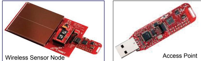
Figure 2: Wireless Sensor Node and Access Point for the Experiment
