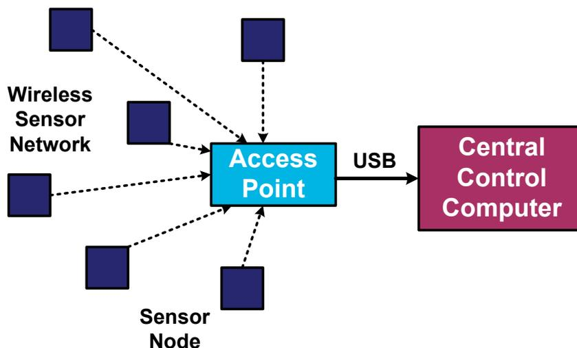
Figure 1: WSN System Architecture for Building Environment Monitoring
