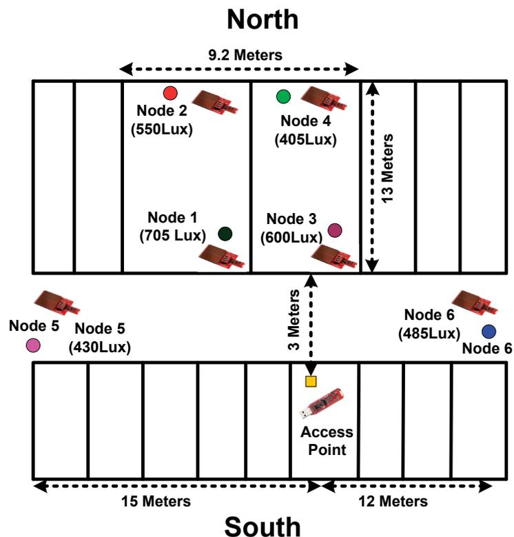
Figure 3: Wireless Sensor Node System Floor Plan
