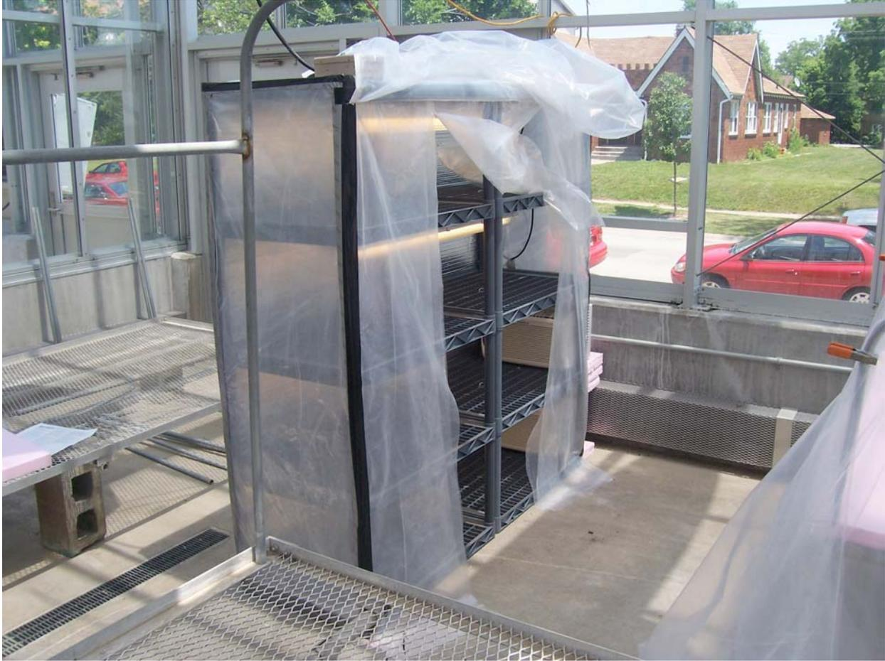
**Figure 1. The completed air-conditioned plant shelf, with the two layers of clear plastic peeled back.**
