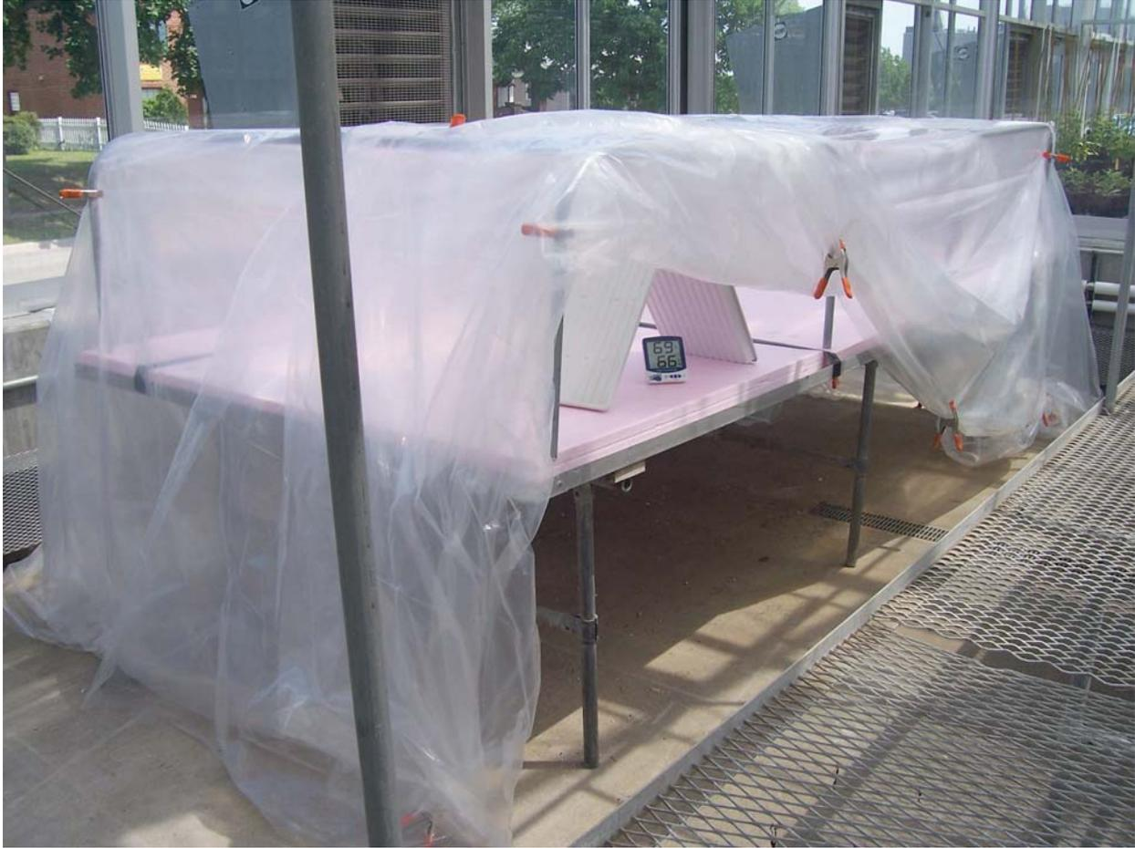
**Figure 3. The completed air-conditioned plant bench, with the two layers of clear plastic peeled back.**
