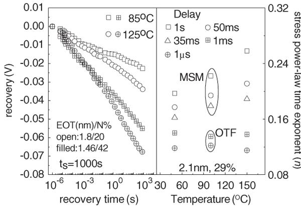
Fig. 4. (LHS) Time evolution of recovery at different  $T$ 's for devices having different EOTs and  $N\%$ 's at  $E_{OX,S} \sim 8.5$  MV/cm and  $E_{OX,R} \sim 3.5$  MV/cm. (RHS) Power-law time exponent (10–1000 s) as a function of stress  $T$  obtained from MSM, OTF, and UF-OTF measurement techniques under different delays at constant  $E_{OX} \sim 8.5$  MV/cm during stress.
