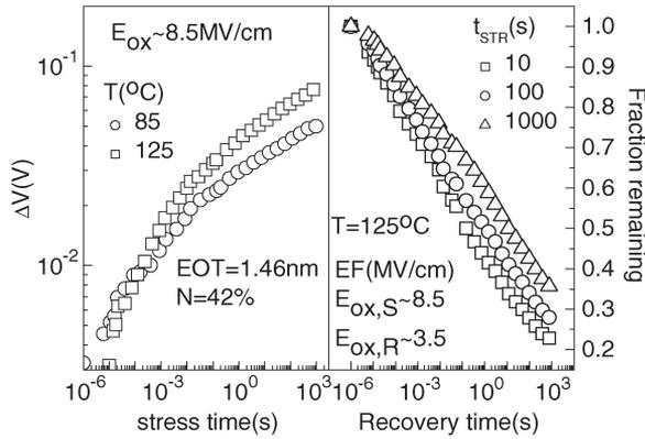
Fig. 1. (LHS) Time evolution of the measured  $\Delta V_T$  at different  $T$ 's but constant  $E_{OX}$  during stress, and (RHS) time evolution of the fractional degradation remaining during recovery for different stress times at constant  $T$  and poststress  $E_{OX}$  for a 1.46-nm EOT and 42% N device.
