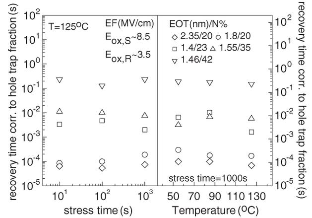
Fig. 3. Time during recovery corresponding to hole-trap fraction as a function of (LHS) stress time at constant  $T$  and (RHS) stress  $T$  at constant stress time for devices having different EOTs and N%'s. This time is defined as hole-detrapping time during the early-recovery phase (see the text).
