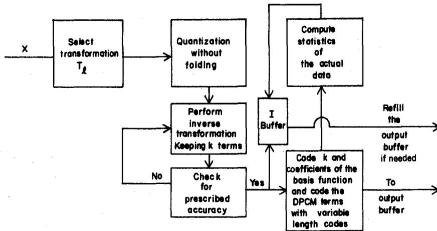
Figure 1. Simplified Block Diagram Showing the Adaptive Error Control System
