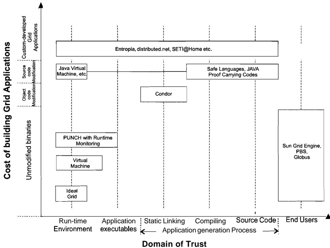
**Figure 3.2. Classification of Grid Environments**
