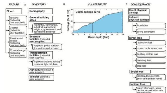
**Figure 4.** Schematic Representation of Hazards, Inventory, Damage Functions, Risks in Hazus. Source: Nastev & Todorov, 2013
