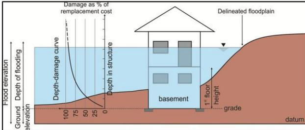
**Figure 5.** Schematic representation of the hazard parameters for a typical Canadian house with a basement [1st floor in Hazus] Source: Nastev & Todorov, 2013
