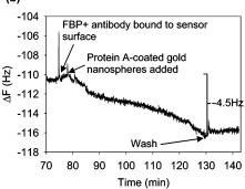
Figure 5. Folate binding protein signal amplification using antibodies against FBP (anti-FBP) and protein-A-coated gold nanospheres. (a) FBP (30 nM) was added to the system, followed by subsequent additions of anti-FBP antibody and protein A nanospheres. PBS washes were performed between steps. (b) Detection of 50 pM FBP using antibody/protein A nanosphere signal enhancement.
