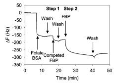
**Figure 4.** FBP detection in the presence of serum. Competed FBP injection (1000 nM FBP in the presence of 100-fold excess free folic acid) revealed an  $\sim$ 30-Hz signal due to nonspecific binding, whereas addition of noncompeted FBP (1000 nM) led to a signal change of 120 Hz.
