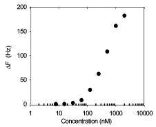
**Figure 3.** Binding of FBP to folate BSA on QCM surface at varying FBP concentrations (7.5 nM to 2  $\mu$ M).
