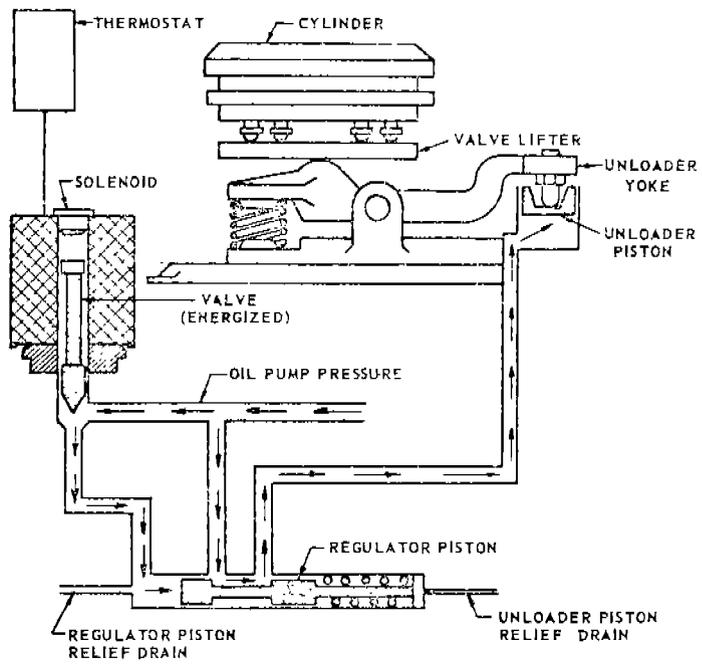
**ELECTRIC UNLOADER MECHANISM**
