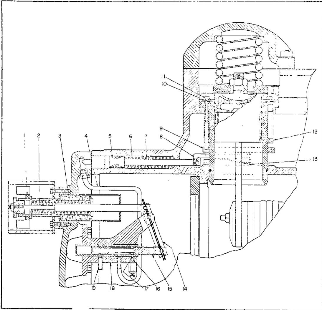
SLIDING YOKE AND RAMP UNLOADER WITH SUCTION
