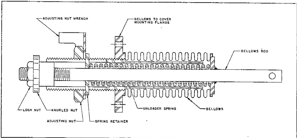
UNLOADER BELLOWS AND SPRING ASSEMBLY
