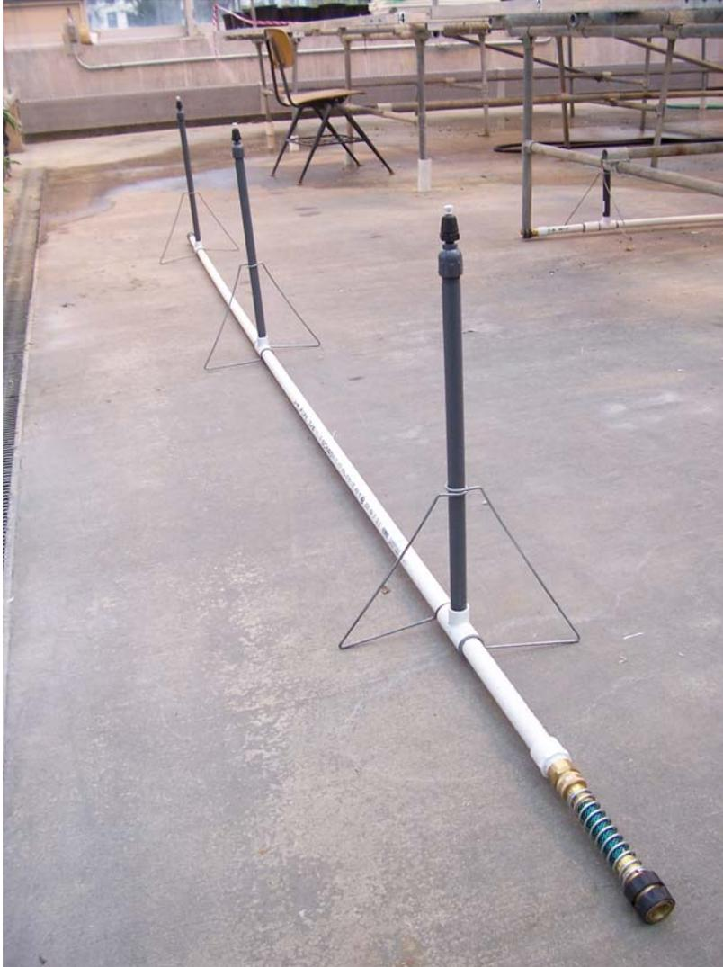
**Figure 2. PVC mist system. The system uses commercially available nozzles and supports, with other parts bought at hardware store. This system is portable and storable. It requires a irrigation timer attached to hose spigot.**
