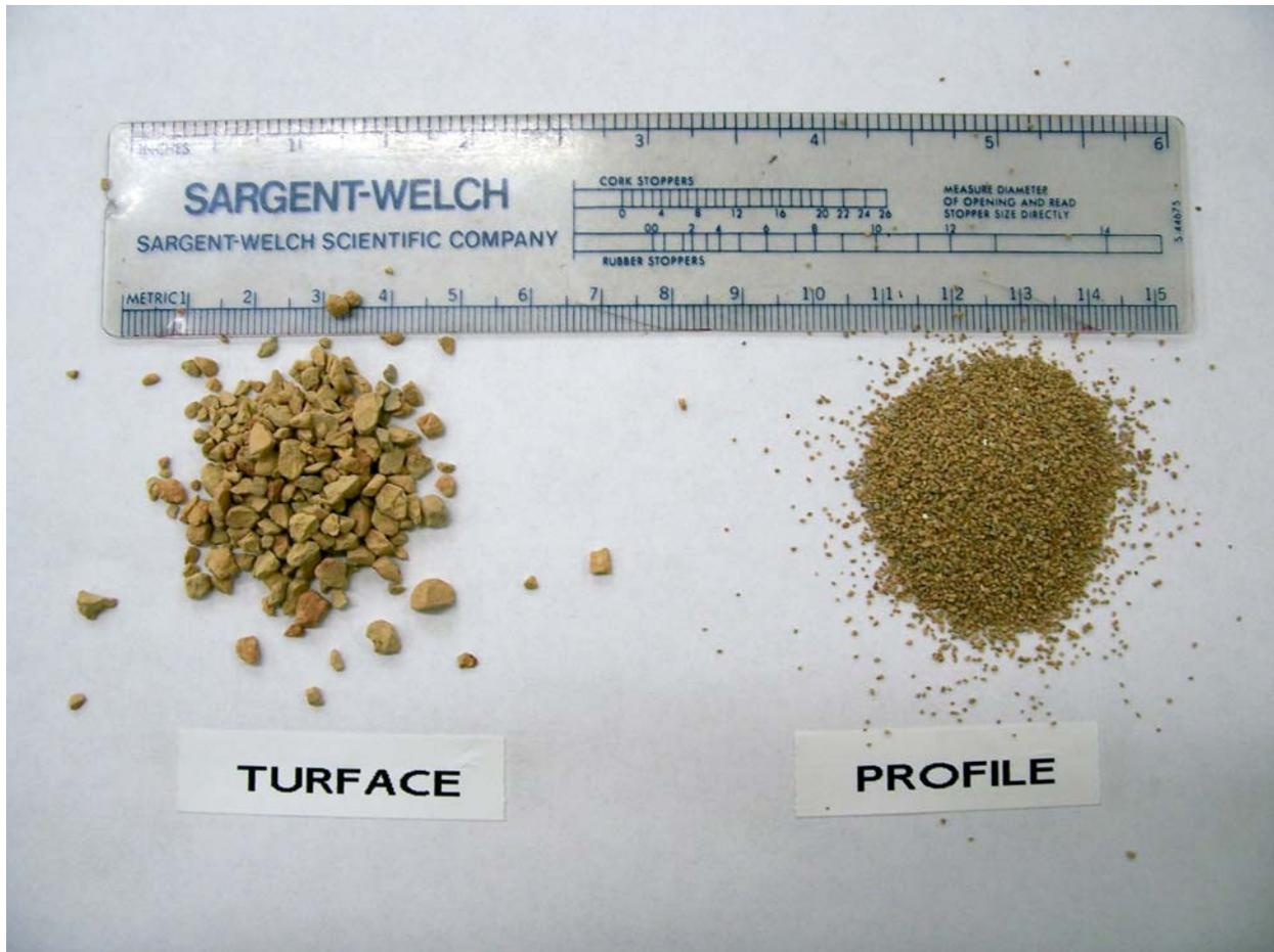
**Figure 4. Turface MVP and Profile Greens calcined clay granules. These products are manufactured for athletic fields and golf course industry to improve drainage.**
