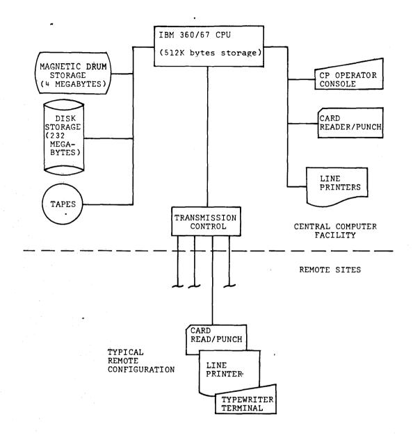
Figure 1. The System Hardware Configuration.
