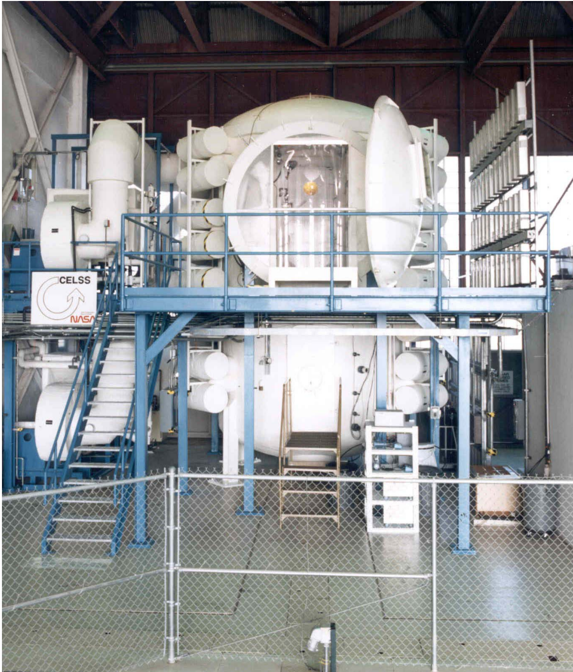
Figure 2. BPC located at Hangar L at KSC, FL (front view, 1986). The chamber provided a closed atmospheric volume of about 113 \text{ m}^3 (including air ducting) with 20 \text{ m}^2 of crop growing area. External nutrient solution tanks were not in place at the time of this photo.
