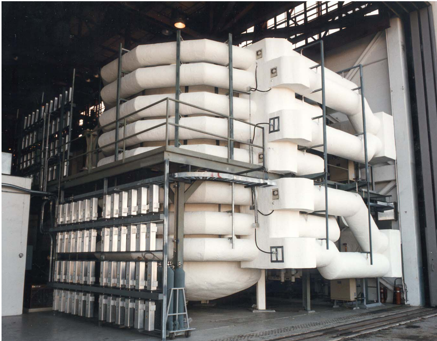
Figure 3. BPC located at Hangar L at KSC, FL (rear view, 1986). Banks of ballasts for the 96 400-W high-pressure sodium (HPS) lamps are visible at the left. Construction began on the chamber in 1985, with operational capabilities completed for most subsystems by 1988.
